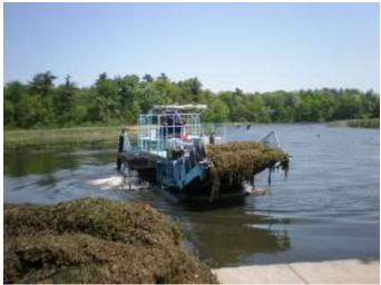
Figure 50: Aquatic Plant Harvester on Rice Lake, WI
