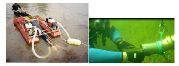
Figure 49: DASH Diver Assisted Suction Harvest (Aquacleaner Environmental, http://www.aquacleaner.com/index.html); Many Waters, LLC)
