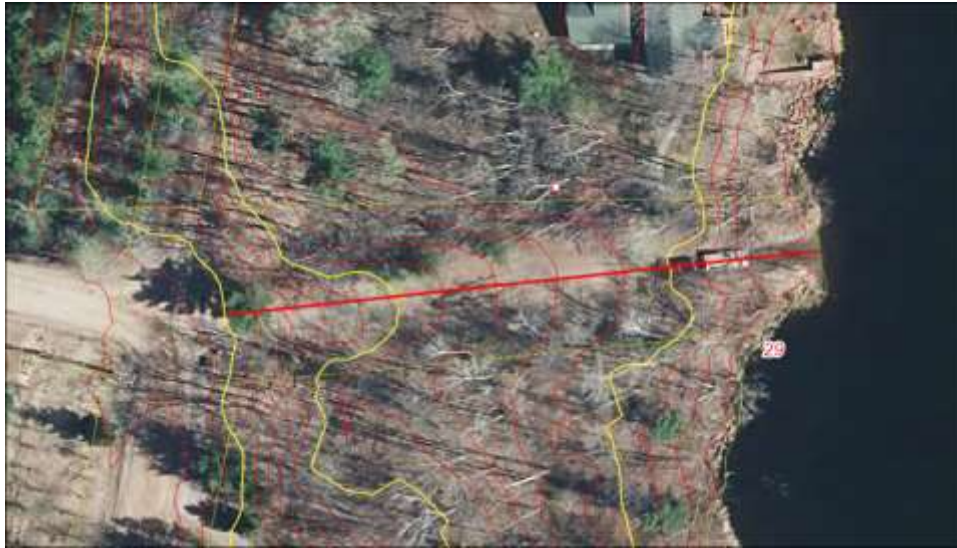
Figure 17: Lakeland Township boat landing on the west side of Granite Lake – 2-ft (red) and 10-ft (yellow) contours. Red line is 300-ft long.
