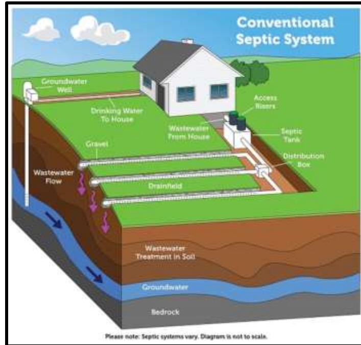
Figure 40: Diagram of a conventional septic system and drain field
