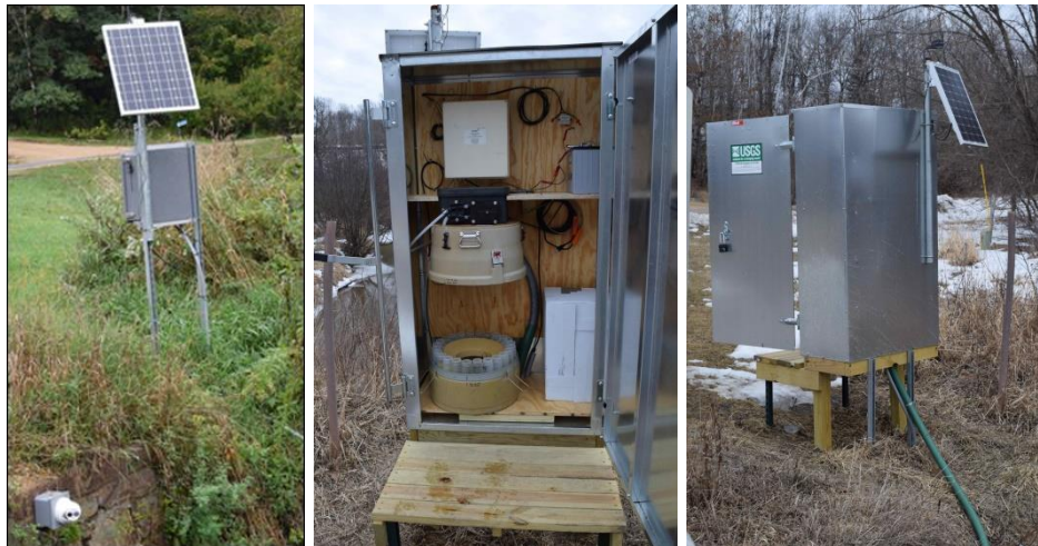
Figure 33: Camera installation for “camera image stage-interpretation” (left) (K. Keegstra, 2019); Typical USGS recording streamflow-gaging station with automatic water sampler for load determinations (middle & right) (K. Keegstra, 2021)
