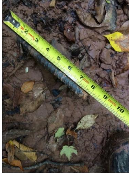
Figure 43: Erosion pin inserted into a streambank showing 8” of soil eroded after inspection in Kankapot Creek, Calumet County, Wisconsin.
