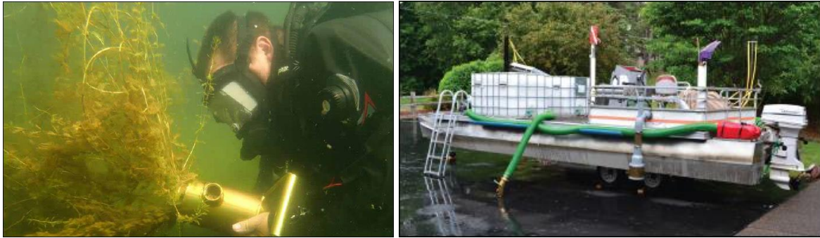
Figure 27: DASH – Feeding EWM into the underwater Suction Hose (Marinette Co.); and a sample DASH Pontoon Boat (Beaver Dam Lake Management District)
