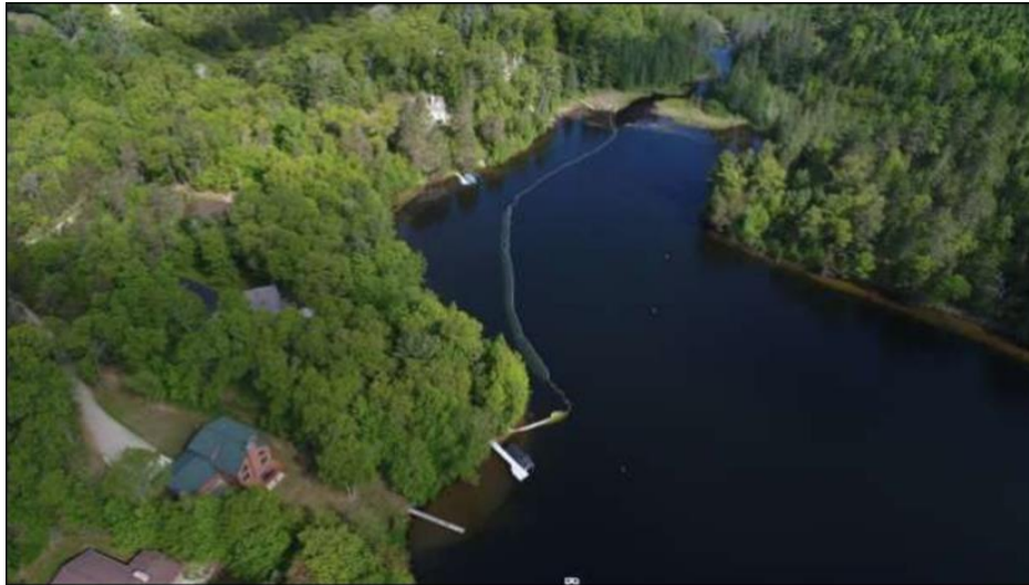
Figure 41. Limno-curtain installed on Thunder Lake (photo from Marinette Co. LWCD)
