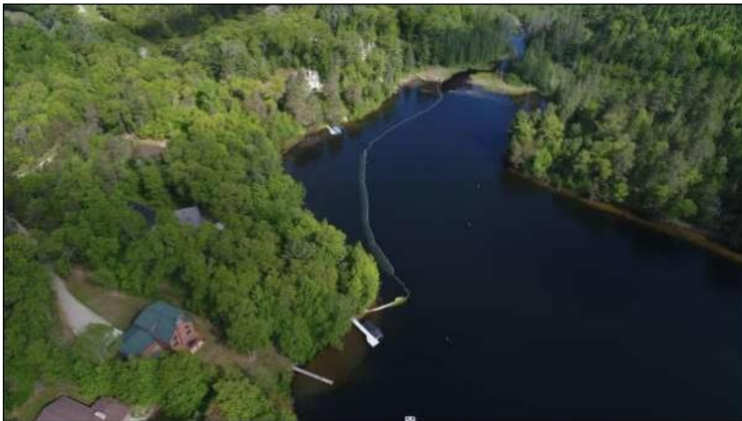
Figure 39: Limno-curtain installed on Thunder Lake (photo from Marinette Co. LWCD)
