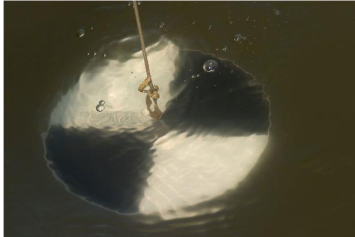
Figure 7: Black and white Secchi disk
